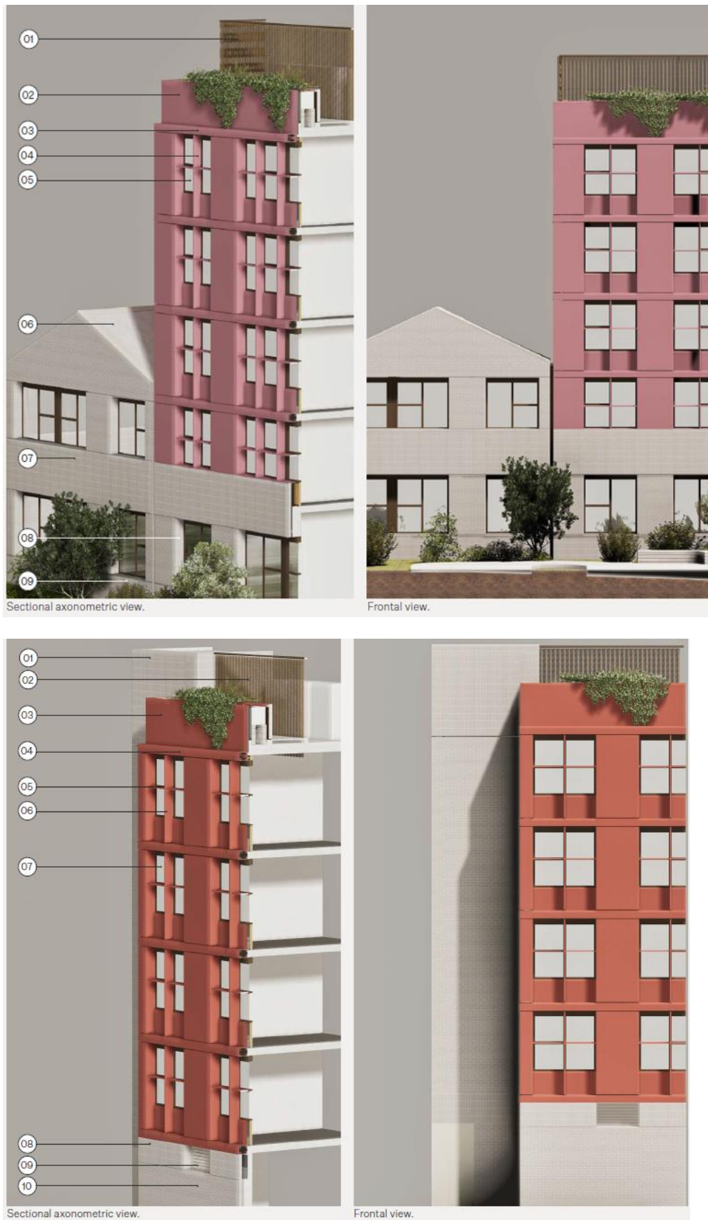
Figure 32: Facade details to manage solar access
